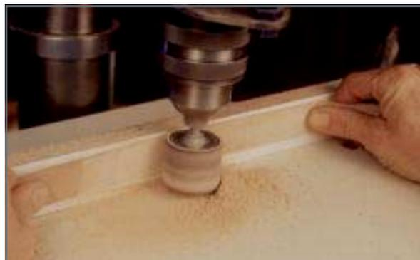
Photo #6: Sanding leather thickness
